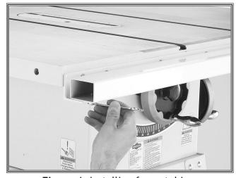
Figure 4. Installing fence tubing.
